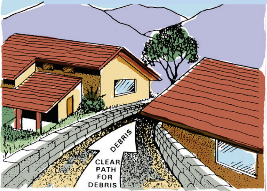
Figure 6: Directing Debris Flows Between Buildings – How to channel debris through and away from buildings.
